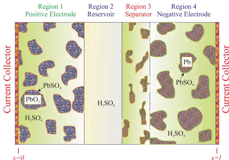
Figure 1: A typical model of lead–acid cell.
