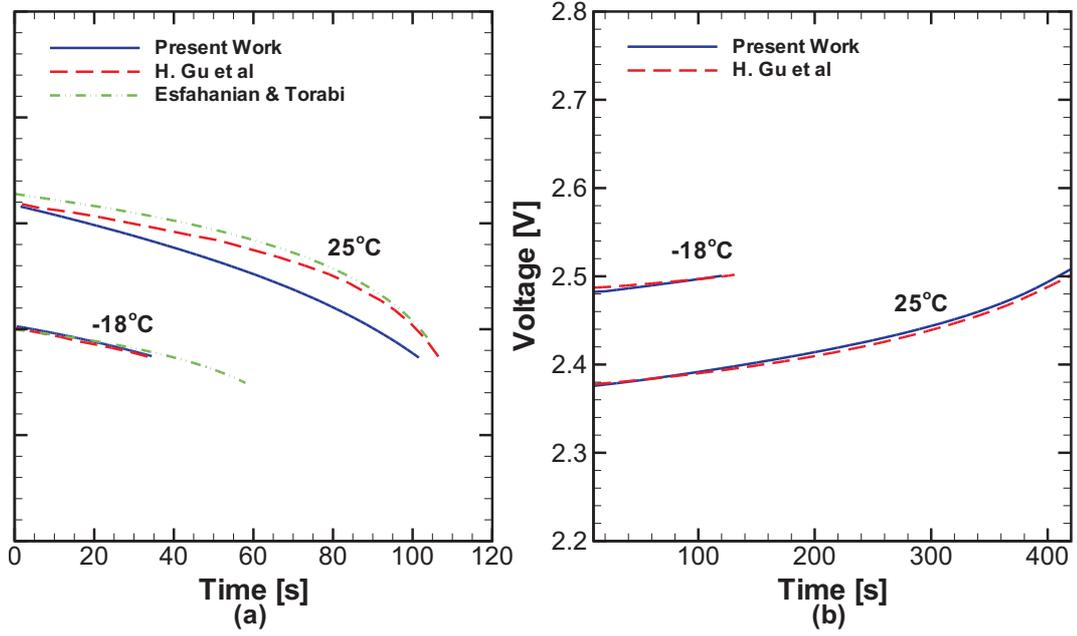
Figure 5: Variation of cell voltage vs. time of cell II at (a) Discharge and (b) Charge.
