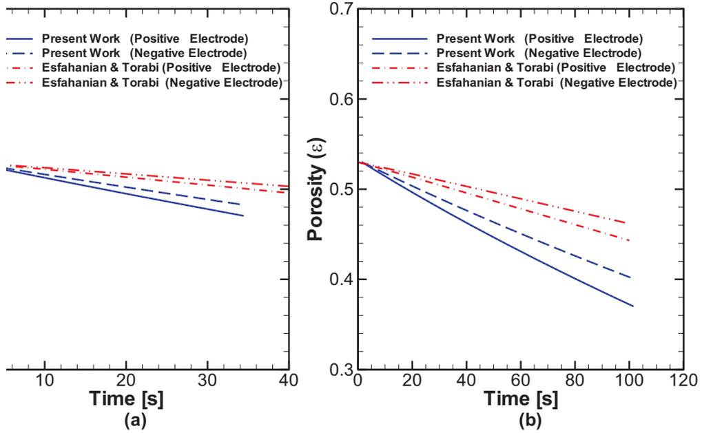
Figure 7: Variation of electrode porosity of cell II vs. time at (a)  $T = -18\text{ }^{\circ}\text{C}$  and (b)  $T = +25\text{ }^{\circ}\text{C}$ .
