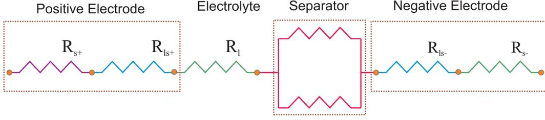
Figure 2: Resistance model of lead–acid cell.
