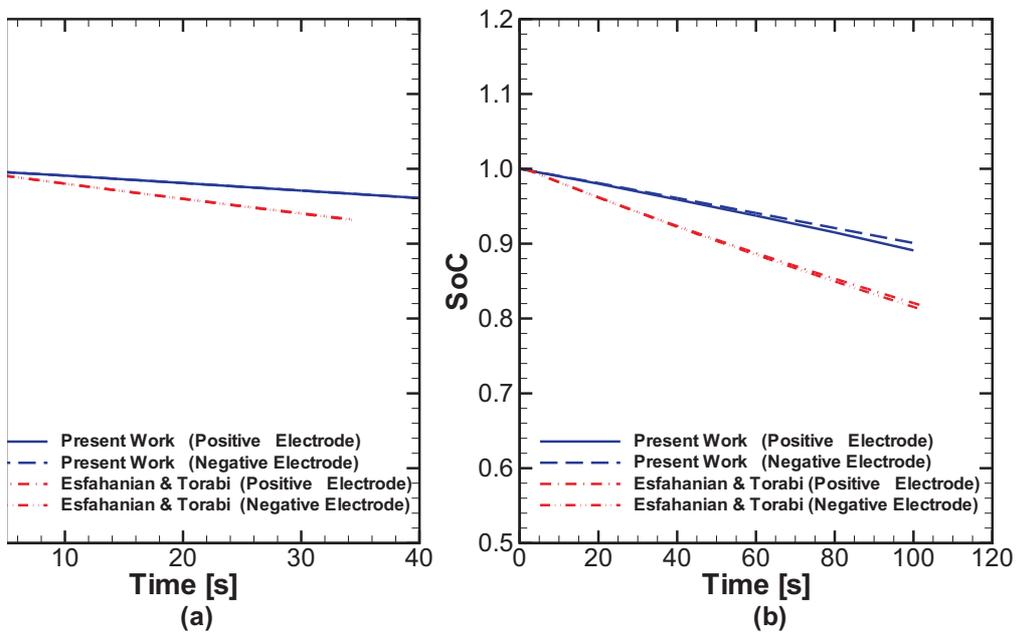
Figure 8: Variation of SoC of cell II vs. time at (a)  $T = -18\text{ }^{\circ}\text{C}$  and (b)  $T = +25\text{ }^{\circ}\text{C}$ .
